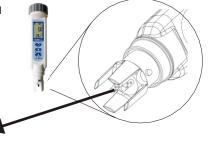
To reduce the air bubbles, dip the electrode completely and swing in air to get rid of bubble
